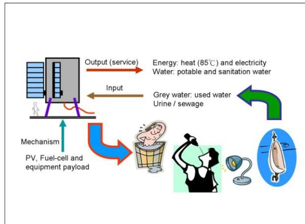
Figure 7. System scheme of S-RRV
