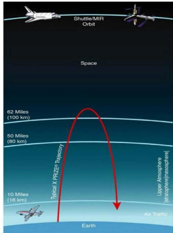
Figure 1. Concept of sub-orbital flight (courtesy of XPrize homepage)
